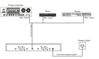
1)The power supply is connected to the power jack of the receiver.
