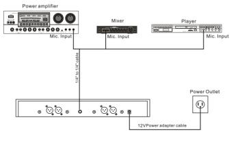
1)The power supply is connected to the power jack of the receiver.
